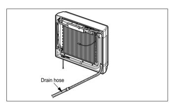
2. Tape the tubing, drain hose and the connecting cable. Be sure that the drain hose is located at the lowest side of the bundle. Locating at the upper side can cause drain pan to overflow inside the unit.
